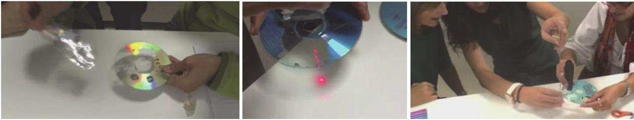
Figure 1. Participants in a teacher training workshop peel off the reflecting layer, study the diffraction phenomenon and perform the measurements needed in order to calculate the grating period.
