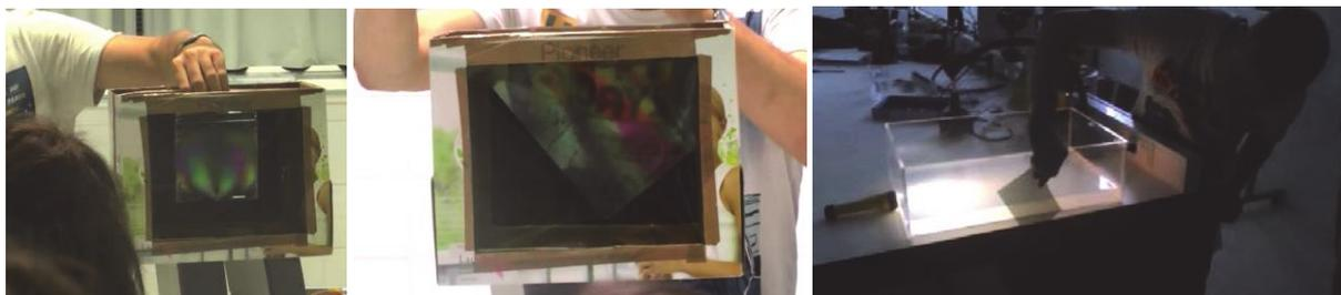
Figure 5. Polarization experiments: visualization of the mechanical tensions in a CD plastic case with a polariscope (left), illustration of the birefringence properties of an acetate transparency acting as a half-wave plate (center), and study of the polarization of scattered light (right).
