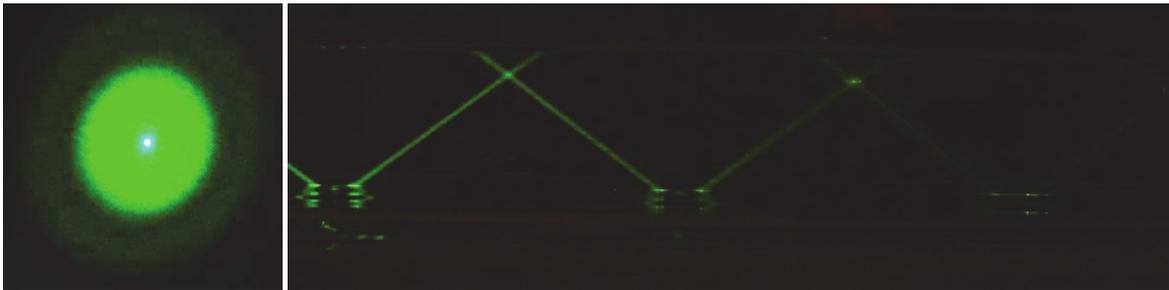
Figure 4. Airy disk pattern created with a laser and a blood sample (left) and total internal reflection in a water tank (right).
