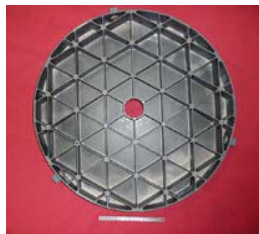
Figure 7. Telescope primary mirror made of SiC
