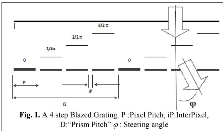
$2\pi$  retardation device is assumed and  $q$  represents the number of steps in the pattern) ignoring any loss originating in the interpixel space [3]. Assuming a reflective device capable of introducing a phase difference of minimum 1064nm per path, a deviation of  $\pm 2^\circ$  at 1064nm can be achieved with pixel pitch sizes in the order of  $7.5\mu\text{m}$ , using a 4 step sawtooth pattern.
