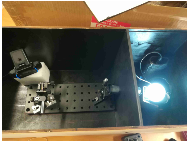
Figure 4. A picture of the spectrometer showing (from left to right) the source, hollow passage, adjustable slit on the optical breadboard, the transmission grating mounted on the optical breadboard and the webcam at roughly 40° from the optical axis. The chamber containing the source is covered with a transparent acrylic slider (not shown) and the optics chamber is covered on the top by a wooden slider to make it light tight.
