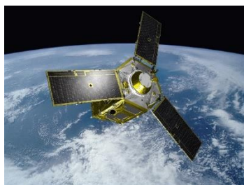
Figure 1. The Pléiades satellite and its focal plane array. The use of multiple folding mirrors to reduce the size of the image greatly complexifies the focal plane and its integration.
