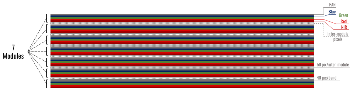
Figure 3. Schematics of the detector used in our design.
