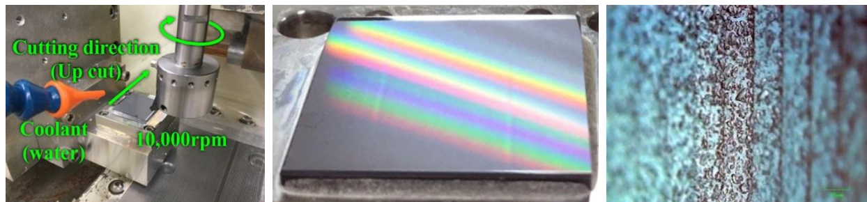
Figure 11 Fabrication of Si grism grating by fly cutting (left), Si grism for MIMIZUKU (middle) and microscope photograph of grooves (right).
