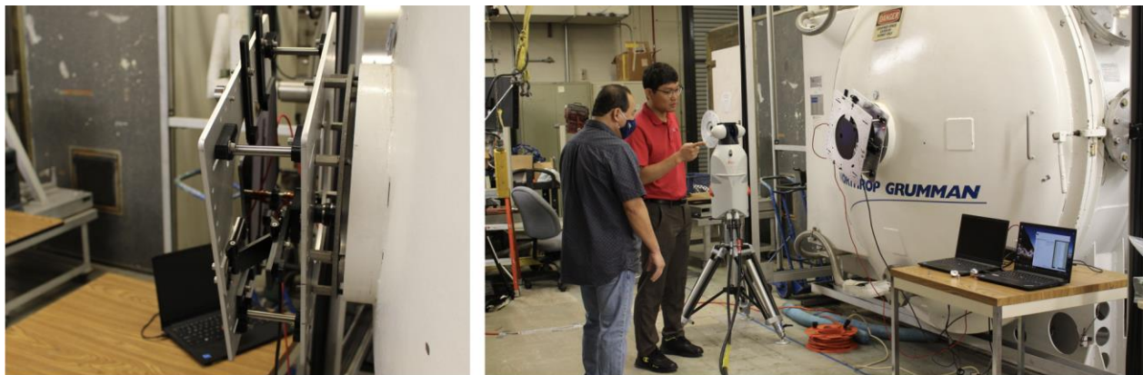
Figure 8. The deflectometer frame consists of two 14" x 14" aluminum plates with mounting holes to constrain a camera and illumination screen (left). Standoffs fastened through aluminum slots allow for translation, if required. The plates were fastened to multiple 3/8" bolts standing out from the TVAC clear aperture window. The entire deflectometer assembly is rotated 22 degrees from the normal vector defined at the floor in order to match the orientation of the bolt hole pattern (right).
