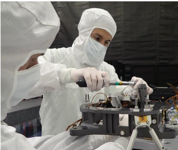
Figure 4. Mounting the mirrors on the SiC Spectro structure
