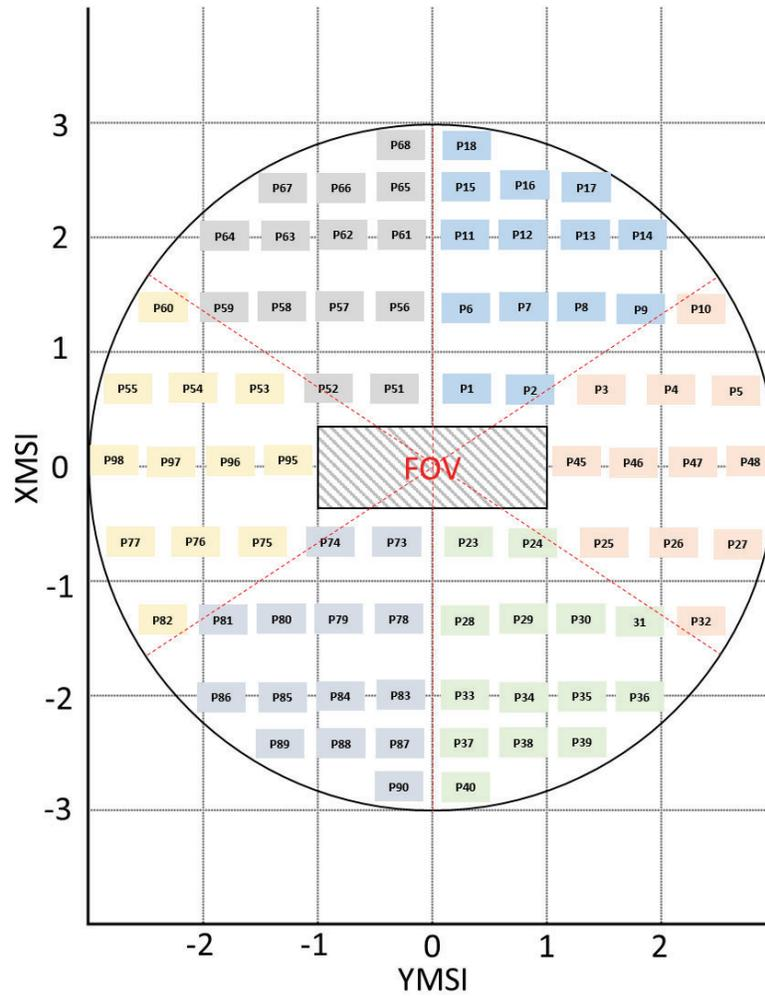
Figure 6 - Positions of the diffusing source out of the field of view
