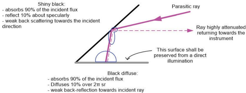
Figure 4 - Principle of the light trap
