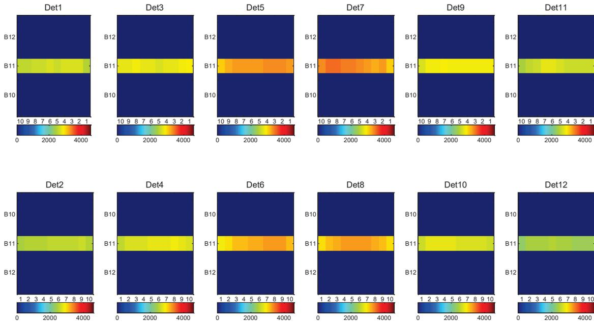
Figure 19 – MSI-D straylight due to the Earth albedo for SWIR band B11
