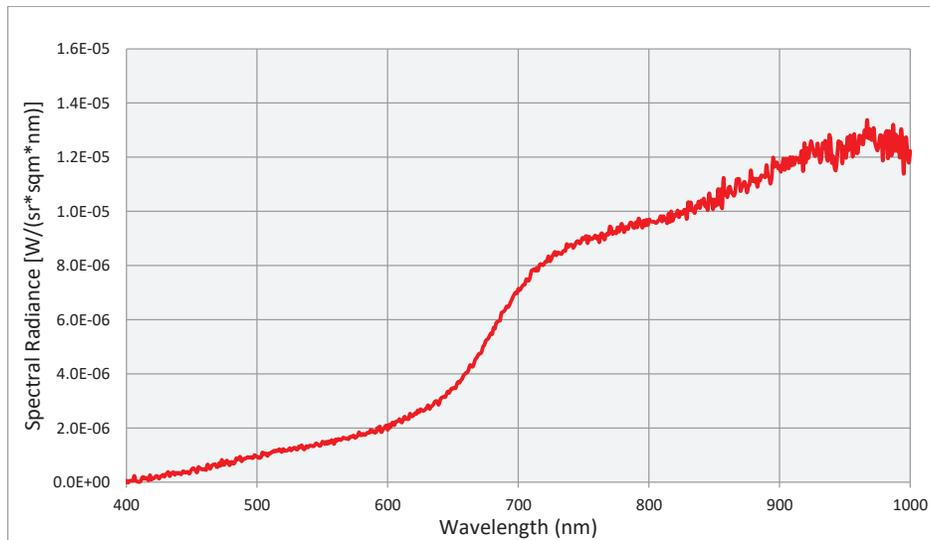
*Figure 12 - Radiance of the light trap (with the diffusing source in direction of the light trap)*
