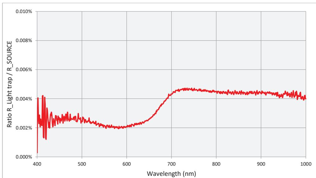
**Figure 14 - Light Trap efficiency: radiance of the light trap / radiance of the source**
