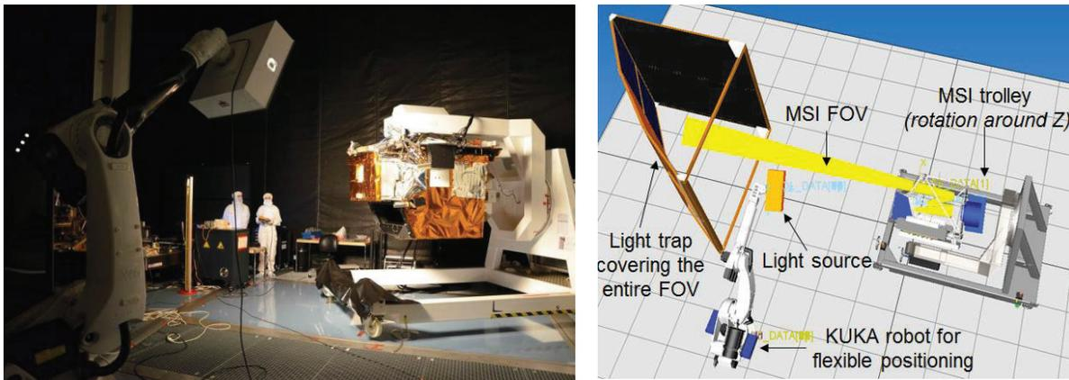
Figure 5 – Overview of the straylight setup
