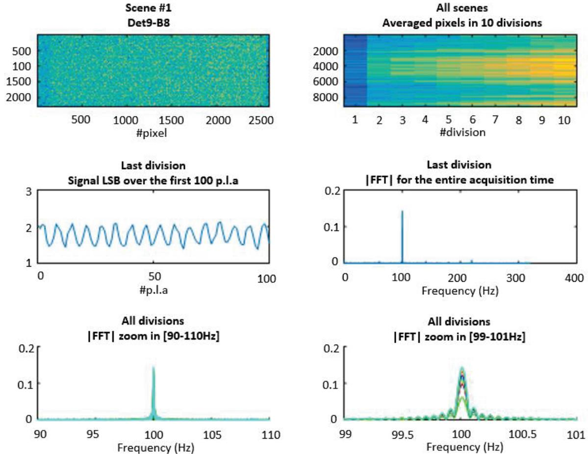
*Figure 8 - Example of FFT processing with straylight*
