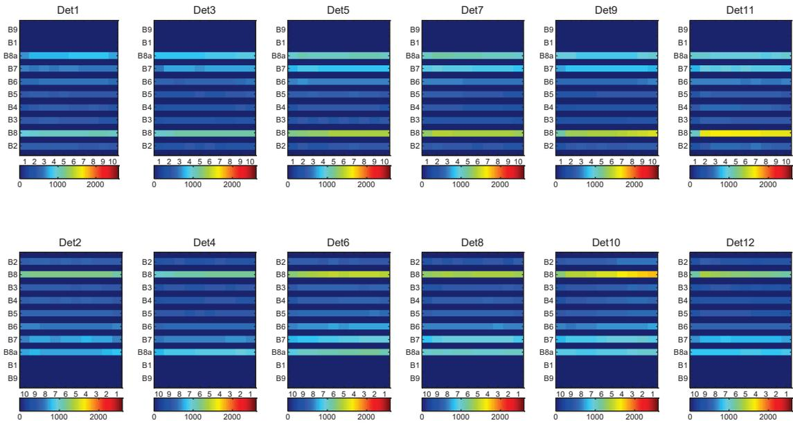
Figure 18 – MSI-D straylight due to the Earth albedo for VNIR bands
