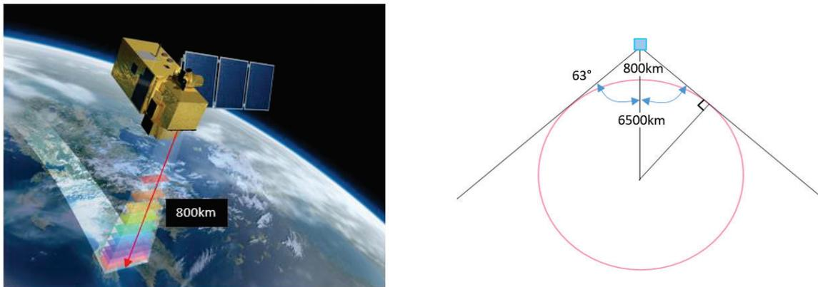
*Figure 3 - The Earth is seen from the telescope under a field of view of  $\pm 63^\circ$*
