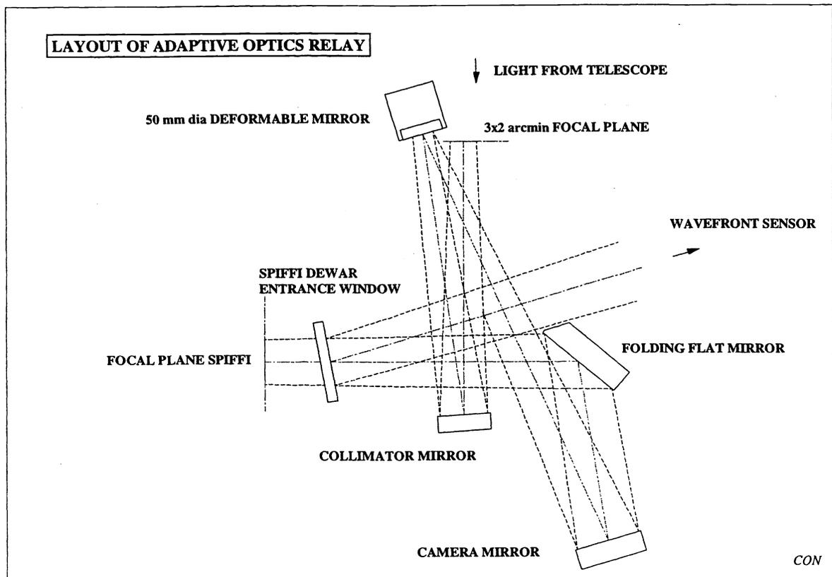
**Figure 4.** Optical layout of the MACAO relay optics, from the VLT Cass focus to the SPIFFI cold focal plane. The SPIFFI dewar window acts as a dichroic to send the visible light to the WFS.  $2 \times 3$  arcmin of field are transferred, to allow for NGS selection
