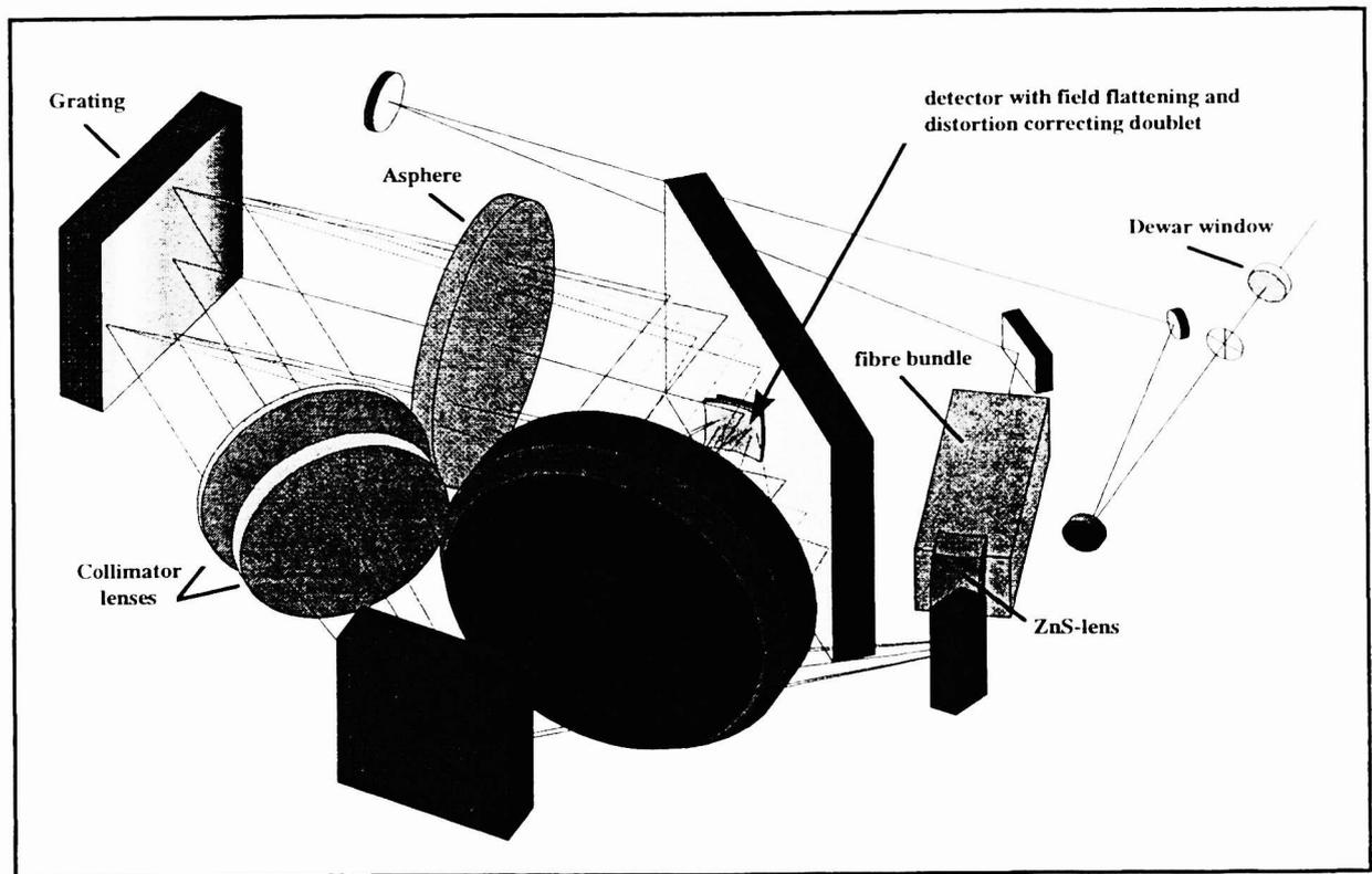
**Figure 2.** Perspective view of the SPIFFI spectrometer optics. The fiber slicer is shown schematically as a box which rearranges the hexagonal input field to a long slit. The dewar entrance window also serves as a beam splitter.
