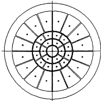
Figure 3. Layout of the 35 element wavefront sensor, with the APDs centered on each lenslet element
