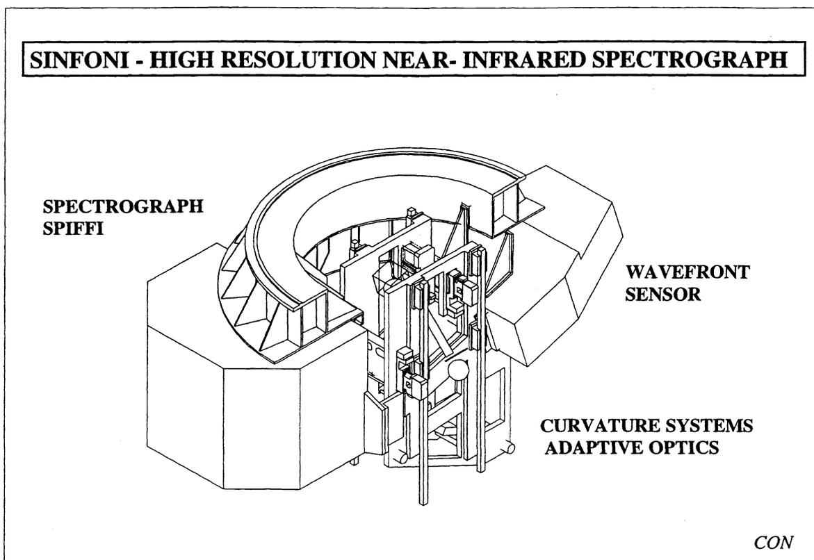
**Figure 5.** Two views of the MACAO optomechanics, for the main optical relay optics. A field of  $2 \times 3$  arcmin in the  $f/13.4$  input beam is transferred to the  $f/17$  cold focal plane of SPIFFI. The SPIFFI entrance window also acts as a dichroic to separate the visible light, reflected toward the WFS, from the NIR light.
