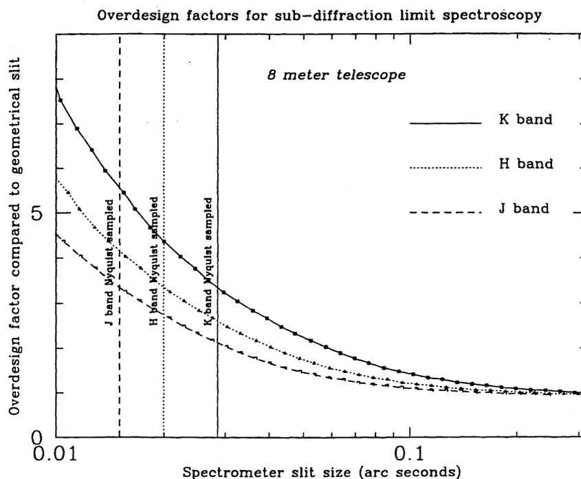
**Figure 1.** Plot showing the over design factor required for a spectrometer to take into account the effects of slit diffraction. The curves show the factor by which the pupil stop must be oversized to include 90% of the energy from the telescope. Results refer to a one dimensional calculation.
