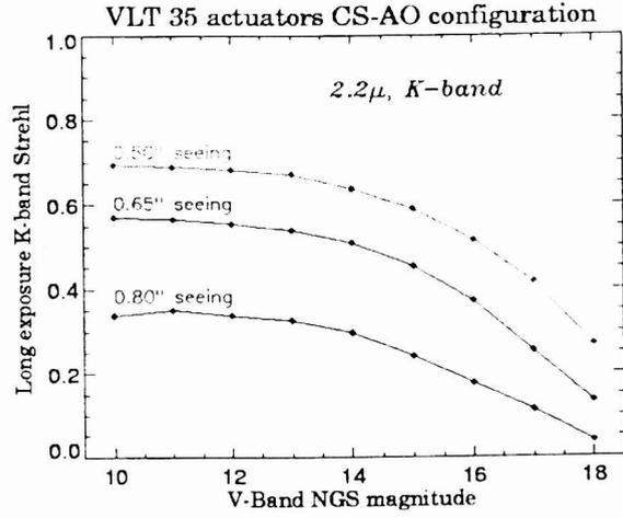
**Figure 8.** NGS K-band Strehl performance of MACAO for different seeing conditions, Paranal model atmosphere. NGS is on-axis.
