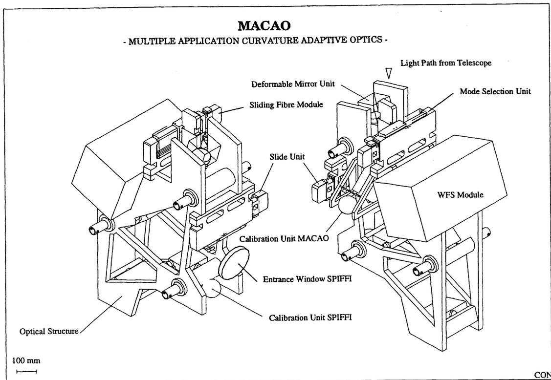
Figure 6. SINFONI mechanical interface, hosting SPIFFI and MACAO. SINFONI attaches directly to the Cassegrain Rotator Adaptor of the VLT.
