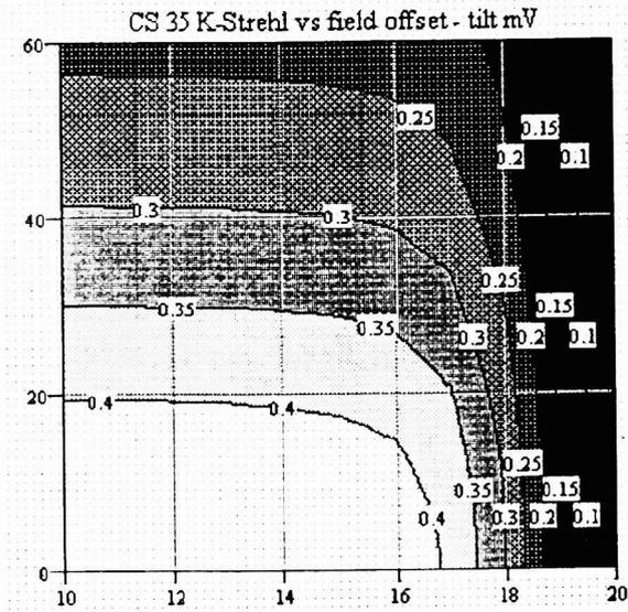
**Figure 9.** Iso-Strehl ratio curves, obtained with a 4.3 W LGS. The y-axis represents the tilt NGS distance from the target, in arcsec. The x-axis represents the tilt NGS V-magnitude.
