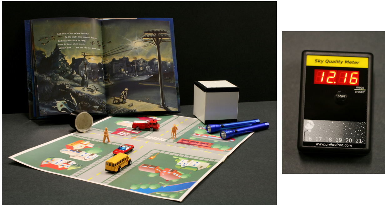
Figure 2. The light shielding demonstration (on the left) and the Sky Quality Meter (on the right).
