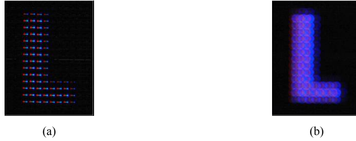
Figure 3. Photographs of LED signs taken by (a) focusing the LED panel and (b) defocusing the LED panel. In this case lamp type LED are located at 20 mm pitch. Black regions between LED lamps are significant when picture was taken by focusing the LED panel. By defocusing the LED panel, the black regions are removed by filling LED lights and smooth shape of L is easily perceived.
