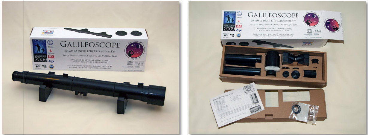
Figure 1: Left: Assembled 50 mm f/10 Galileoscope, on its display stand, which also helps the telescope function as an optical bench for certain types of optics experiments. Right: Unassembled Galileoscope telescope kit. The telescope can be repeatedly assembled and disassembled without tools. It is durable enough for years of classroom use.
