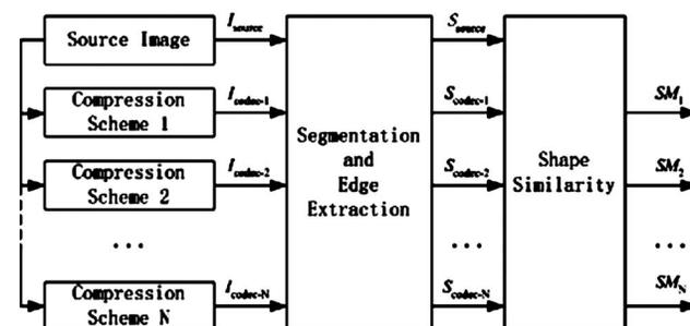
Fig. 1 Diagram of ATR-directed image compression quality evaluation system.
