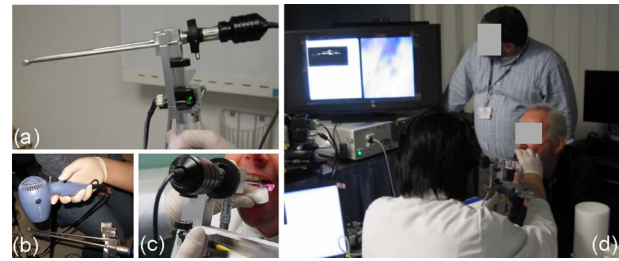
Fig. 2 (a) OCT probe attached to the laryngoscope; (b) defogging before (c) insertion of the probe into pharynx for examination; and (d) dual-channel office-based OCT laryngeal probe in use during laryngeal examination.
