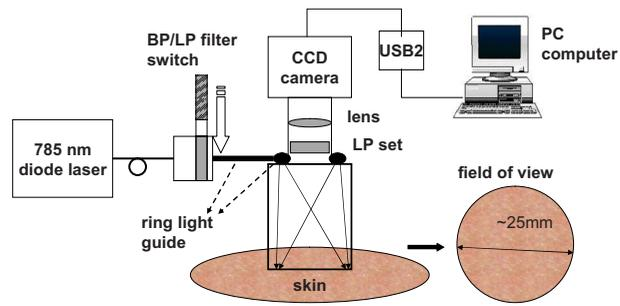
**Fig. 1** Block diagram of the prototype NIR fluorescence imaging system.
