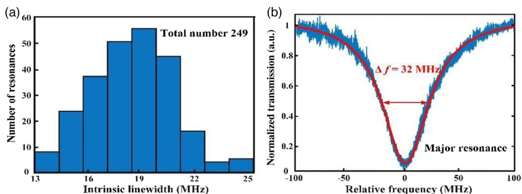
**Fig. 2** (a) The histogram of the intrinsic linewidth of the MRRs; (b) a representative resonance with critical coupling (reproduced from Ref. 4).
