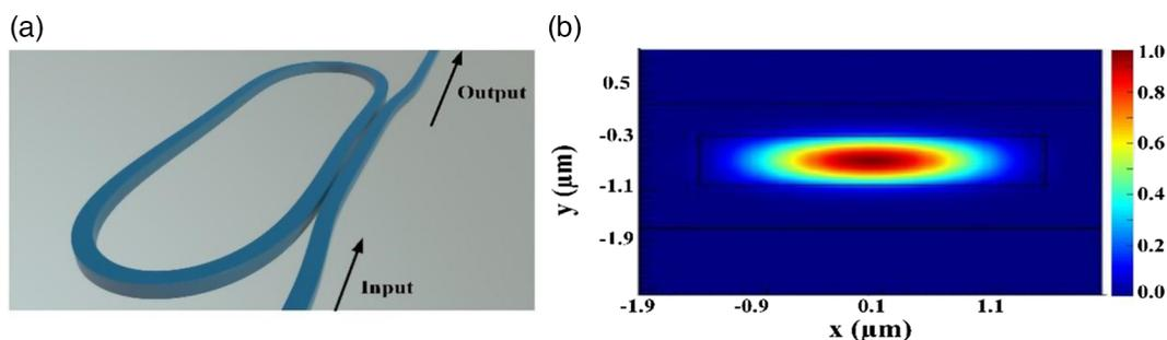
**Fig. 1** (a) Schematic illustration of the proposed compact ultrahigh-Q MRR; (b) the simulated mode profiles when the waveguide width of the MRR is  $3\ \mu\text{m}$  (reproduced from Ref. 4).
