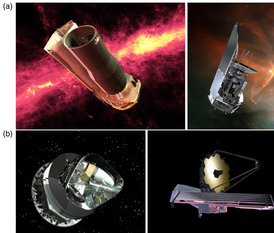
Fig. 6 Four examples of satellites that observe at mid/or far-infrared wavelengths (Sec. 3). (a) Spitzer and Herschel and (b) Planck and JWST, which also use V-groove radiators (thermal shields) to achieve passive cooling up to <40 K.
