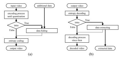
Fig. 4 Flowcharts of the proposed processes: (a) embedding and (b) extracting.
