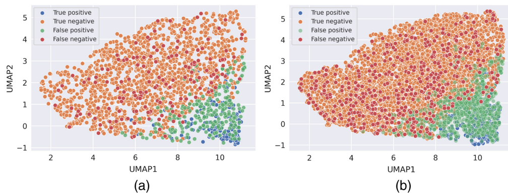
Fig. 10 UMAP visualization of the confusion matrix for (a) the original test set and (b) the current test set. A similar decision variable was chosen by the deep net for both patient cohorts, classifying positive cases from negative cases (division between blue and orange dots). Overall, the model returned a higher percentage of TPs and lower percentage of FPs for the original test set than for the current test set. 12
