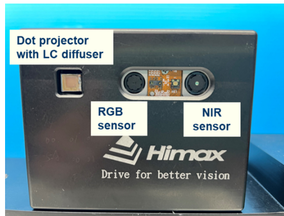
Fig. 2 3D sensing module prototype with two-in-one pattern projector.
