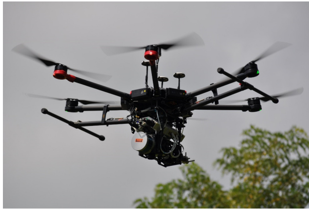
Fig. 3 The MX-1 platform developed by RIT. The Velodyne VLP-16 lidar is visible on the forward end of the peripheral mount at the bottom of the airframe.
