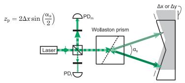
The output angle in the Wollaston prism is typically small, between 0.1 and 2 deg, leading to a straightness sensitivity of between  $\sim 0.005\Delta x$  and  $\sim 0.035 \Delta x$ .
