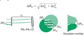
In many cases, the interfering beams have a Gaussian profile. Small walkoff changes cause the overlapping area, and thus the fringe contrast, to significantly decrease.
