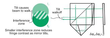
The amount of walkoff scales based on the distance  $z_{\rm n}$  between the interferometer and the target. Even for small rotations, the walkoff can be significant if the distance to the target is large. For small angles, the walkoff is  $\sim 2\Delta\phi/z_n$ , which discounts the additional walkoff that will occur in the beamsplitter and retroreflector. Both tip and tilt will generate walkoff, so the total beam overlap shifts by  $\Delta R_{\phi}$ .
