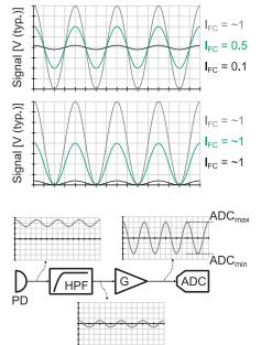
High DC offset leads to varying fringe contrast for different signal amplitudes.
