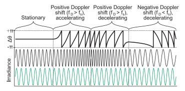
Because the phase change is measured relative to a signal with a defined frequency, there is no directional ambiguity. As long as the phase is correctly unwrapped or fringes are counted, heterodyne interferometers are inherently sensitive to direction.
