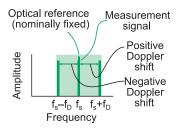
In the **Fourier spectrum**, the optical reference is fixed. When the measurement signal has a frequency lower than the optical reference, the target is moving away from the interferometer because the signal is undergoing a negative Doppler
