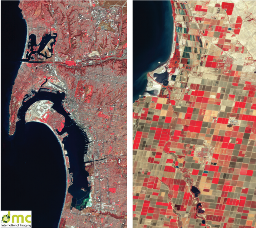
Figure 1.15 Full-frame image captured by the UK-DMC on October 1, 2009 at 17:53:00Z. The false-color “IR” image is 14400 \times 15550 pixels and provides a 30-m ground sample distance (GSD). Regions that appear red have significant healthy vegetation. UK-DMC2 image October 1, 2009, ©2016 DMCii, all rights reserved. Supplied by DMC International Imaging, U.K.
