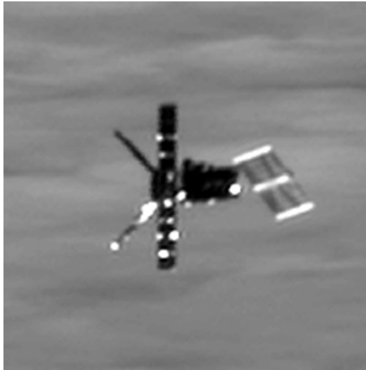
Figure 1.6 On June 3, 2002, SPOT-5 took this picture of the ERS-2 satellite at about 23:00 UTC over the Southern Hemisphere. ERS-2, 42 kilometers below, overtakes SPOT-5 from north-east to south-west at a relative velocity of \sim 81 m/s. Image reprinted with permission of the Centre National d'Études Spatiales (CNES).
