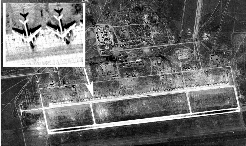
Figure 1.3 Image of the Dolon air base in Chagan, Kazakhstan ( 50^{\circ} 32' 30'' N, 079^{\circ} 11' 30'' E) taken by the Gambit (KH-7) system during Mission 4022 on October 4, 1965. The inset is a close-up of the Tupolev Tu-95 (Bear) bombers along the 4-km runway. North is up. The planes are 46 m in length, with a wingspan of 50 m. The spatial resolution in the scanned image is \sim 0.735 m per pixel. Image reference: DZB00402200056H012001; the film was scanned at a 7 \mu\text{m} pitch. 4
