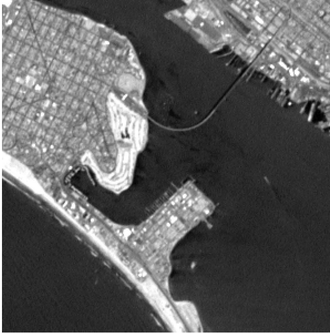
Figure 1.13 Landsat 7 panchromatic channel. The high-spatial-resolution channel for the Enhanced Thematic Mapper Plus (ETM+) has a 15-m resolution capability shown here. The Coronado Bridge starts to appear clearly. The golf course is bright because of this sensor's spectral response extends into the near-infrared (see Chapter 6).
