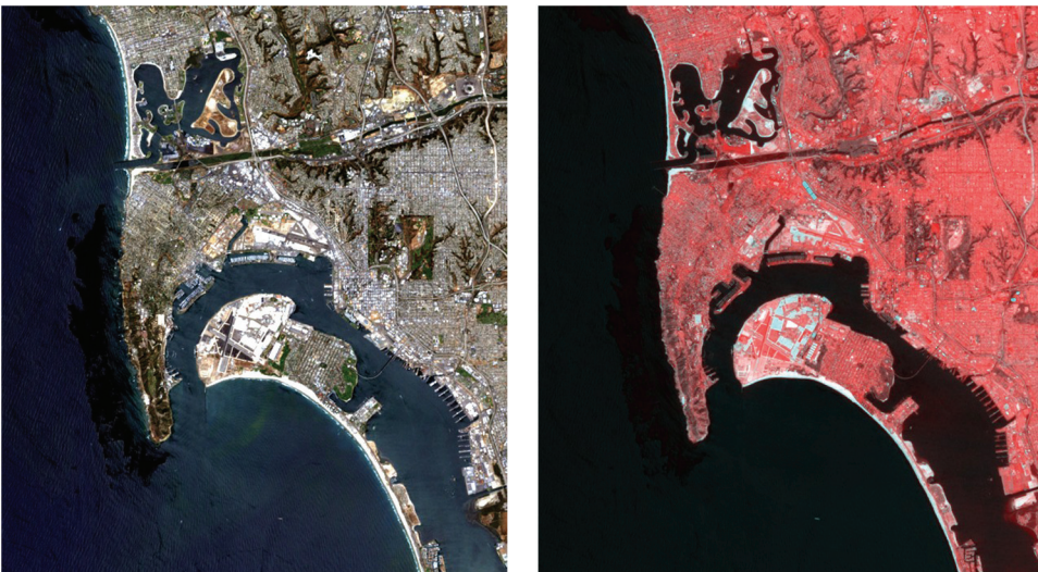
Figure 1.12 Landsat 7 image enlarged (acquired June 14, 2001 at 18:12:08.07Z), with the “true-color” image on the left and a Landsat thermal image on the right. The right image uses IR wavelengths bands 6 and 7; the red is 11 \mu\text{m} , and the green and blue are 2.2 \mu\text{m} .
