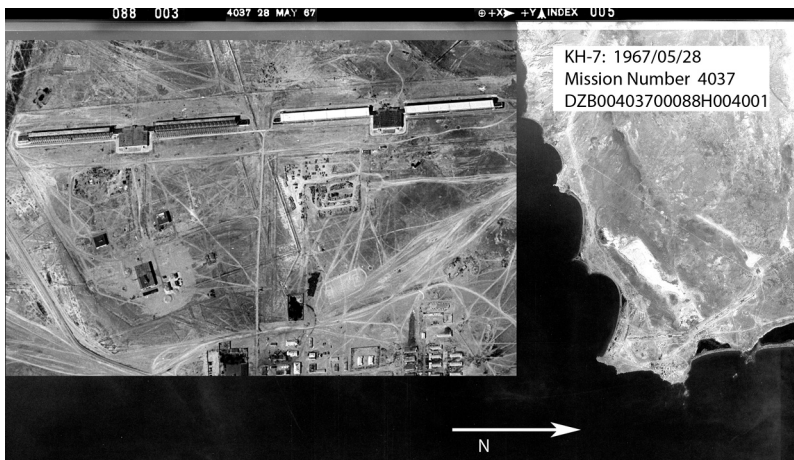
Figure 1.4 This Gambit-1 image shows the Sary Shagan Hen House radar (centered at 46^{\circ} 36' 41'' N, 74^{\circ} 31' 22'' E). The image was taken on May 28, 1967. Similar images with a 1-m resolution date to 1964. These large Soviet radars were designed to watch for ballistic missiles and satellites. The 25-MW system was designed to monitor the south and west with two pairs of antenna, one transmitting and one receiving (bistatic). The image chip for two of the radar systems is overlaid on the full frame image for context. The original film was 9 inches wide (the vertical direction in this frame).
