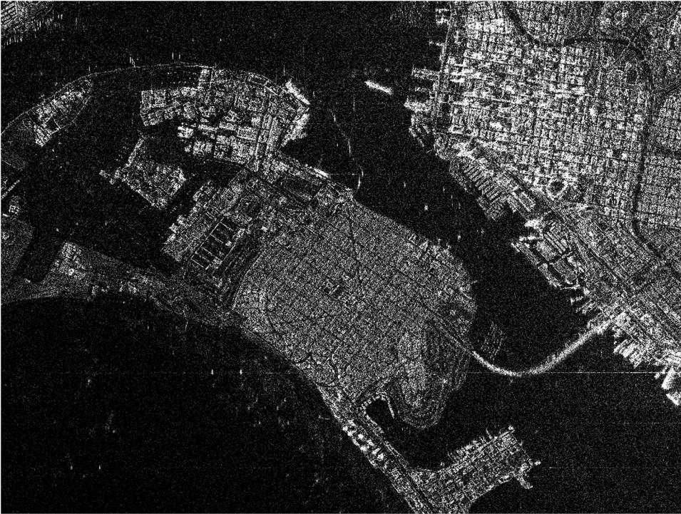
Figure 1.19 RADARSAT-2 image collected at 3-m resolution on 5/5/2009. Polarization is HH. Elements of the scene are well captured by radar, others less so. The Coronado Bridge shows up clearly, as do the air fields due to their absence of reflection. Systems such as RADARSAT-2 have nearly daily access to mid-latitude and high-latitude targets. RADARSAT-2 data © Canadian Space Agency and MacDonald, Dettwiler and Associates Ltd, 2009, all rights reserved.
