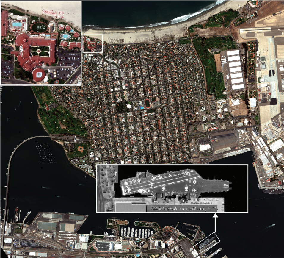
Figure 1.16 Worldview-3 image of Coronado Island, San Diego, California, 9/16/2014. North is approximately to the right, and the sun is to the upper left. The Hotel del Coronado is shown in the upper inset, and the carrier Midway is shown in the lower inset, using the higher-resolution panchromatic data (0.30-m GSD). Imagery reprinted courtesy of DigitalGlobe.
