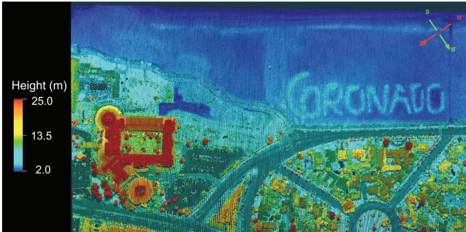
Figure 1.17 Image of Coronado Island, San Diego, California with LiDAR data from USGS. The sensor used was an Optech, Inc. Airborne Laser Terrain Mapper (ALTM) 1225. The LiDAR data were collected on March 24–25, 2006. The following settings were used for these flights: 25-kHz laser pulse rate, 26-Hz scanner rate, \pm 20^\circ scan angle, 300–600-m AGL altitude, and 95–120-kts ground speed.
