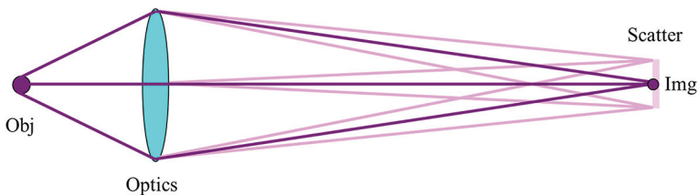
Figure 10.5 Mid-spatial-frequency roughness on the imaging optics causes light to be scattered out of the imaging cone, creating a background halo of illumination.
