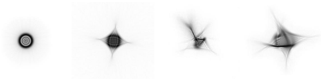
Figure 7-46: PSF at the location of the circle of least confusion for (left to right) spherical aberration, astigmatism, keratoconus, and pellucid marginal degeneration.
