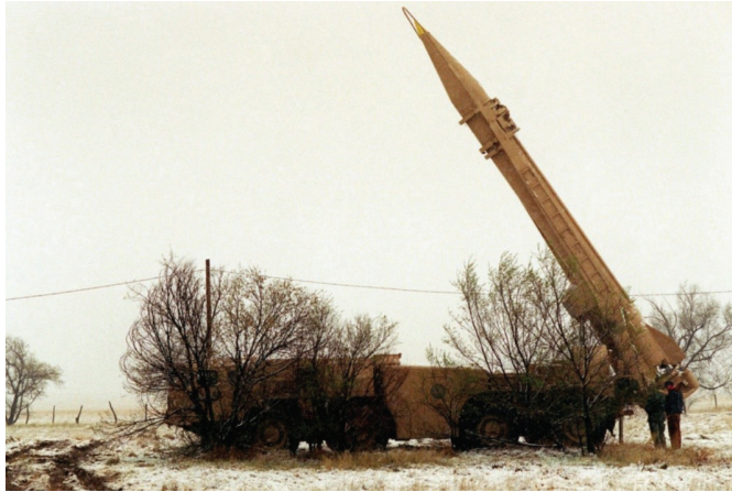
Figure 3.2 Many target types have articulated parts. An ATR must recognize them in all of their variations. The Scud launcher shown here is most dangerous when its missile is in the launch position. (Photo from defense.gov.)
