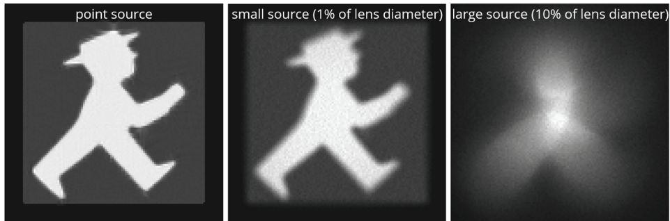
Figure 47 Simulation results for the freeform lens shown in Fig. 39, with varying source size. Left: the nearly perfect result for the point source. Center: the source has a diameter of 1% of the lens, and visible blurring occurs. Right: with the source size being 10% of the lens diameter, the lobes hint at legs, arms and a head, but all details are lost.
